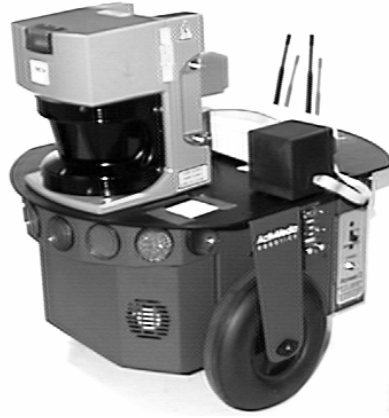
Figure 6.2: A typical Pioneer 2-DX robot. Visible in this image are the two drive wheels, front sonar ring, compass (small cube), Ethernet modem (antennae protruding vertically), and laser range-finder (looks like a coffee-maker). At the rear of the robot is another ring of sonars.
